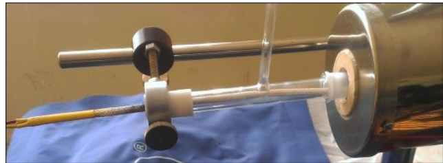
Fig.2. Quartz tube with thermocouple
