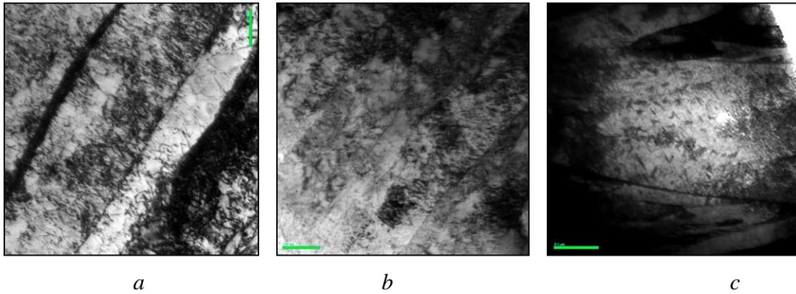
Fig. 1. The microstructure of welded joints produced by laser welding at 880 J/mm (a); 316 J/mm (b, c).
