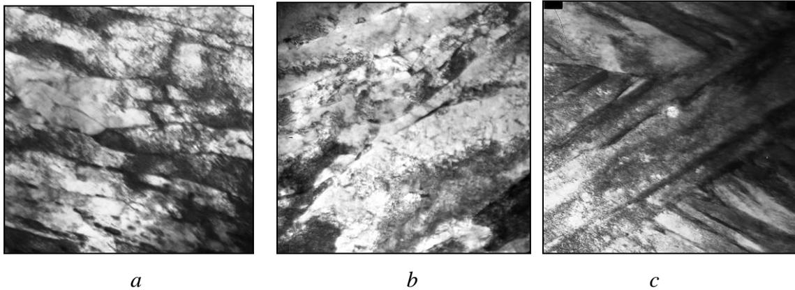
Fig. 2. The microstructure of welded joints produced by hybrid welding at 363 J/mm (a, b); 314 J/mm (c).
