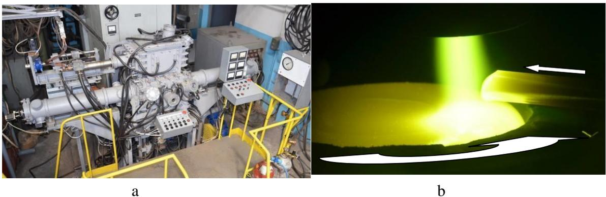
Fig. 4 The newest equipment with computer-controlled unit (a) for the production of single crystals of refractory metals of rotation bodies (b)
