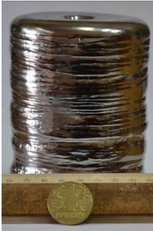
Fig. 5 The appearance of a tungsten crystal with a diameter of 85 mm
