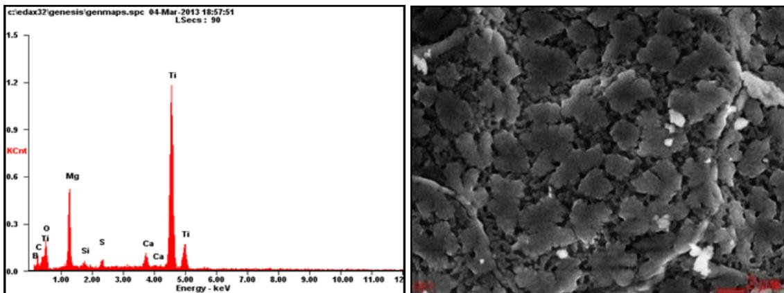
Figure 2 – Microstructure of the composition material on the basis of TiB<sub>2</sub>-TiC- MgO
